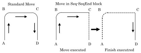
If Finish statement is executed before a robot reaches the point C, a robot moves to the point D without stopping at the point C.
