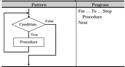
In this figure, "Procedure" may contain not only one step but multiple steps. And it can contain selection structures.
