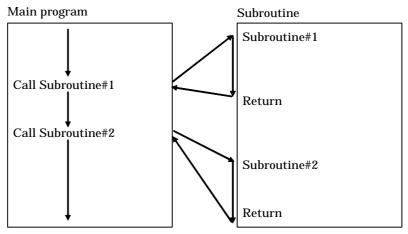
This structure avoids the loss of same procedures in a program. And if the trouble of the procedure happens, only the subroutine has to be modified.
