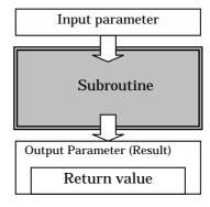
In HrBasic, a local variable is generally used as a parameter to increase the independency of a subroutine.
