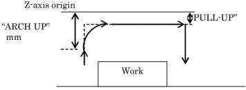
Arch-down-value is the distance of arch-down motion, which is the length from the position of Z-axis origin.
