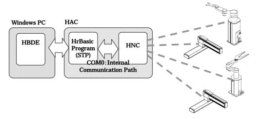
(2) Connection between WinSTP and HNC robot Standardly, WinSTP is connected with HNC by RS-232C interface. HrBasic can communicate with HNC using "COMn" port of PC.
